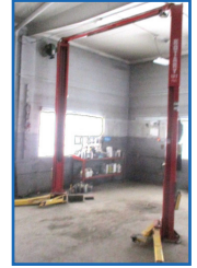
Rotary Lift 9000 lb. capacity model SP0A9-200 ser. AAU0159
