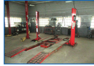
Hunter Engineering twin post drive on alignment lift, model L202 ser. H2P1124P
