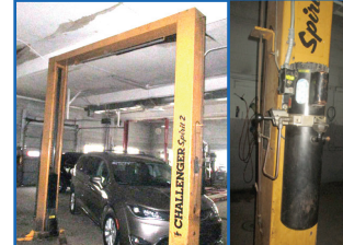
VBM Corporation Challenger Spirit 2 two post 7000 lb. lift, model 31000, ser. 312136
