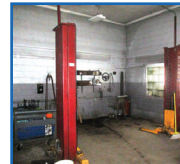
Mohawk 9000 lb. two post lift, model System IA ser. 9704531
